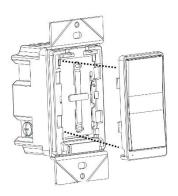
Wire: Strip 10mm (±1) insulation, connect or disconnect for field wiring.
