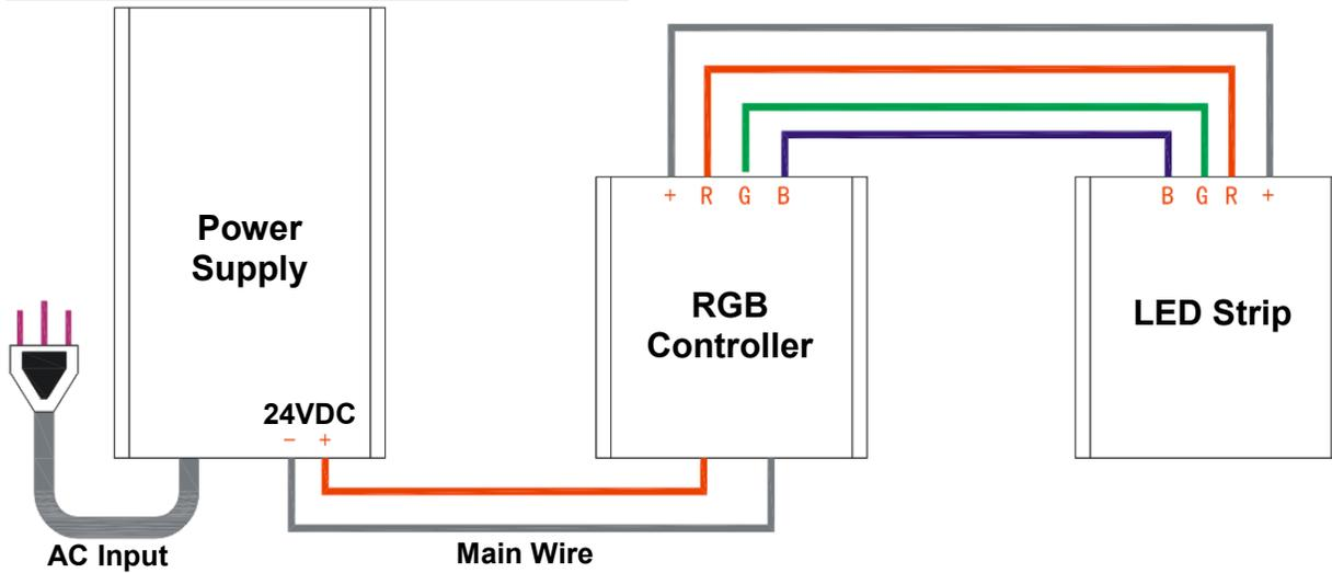
**Note:** For consistent brightness and even appearance, we recommend you to connect the LED strips to a power supply or repeater every 20-30 ft. to minimize voltage drop.
